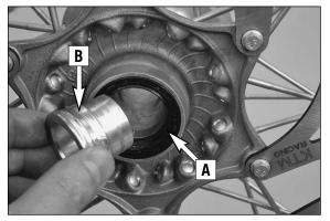
Before remounting the front wheel, clean and grease the shaft seal rings [A] and the bearing surface [B] of the distance bushings and mount the distance bushing.
